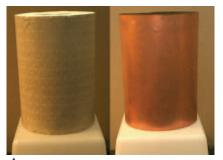
▲ Fig. 6 Cloak (left) and copper cylinder used as a control (right).
