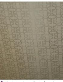
Fig. 4 Outer layer of a simple two-layer cloak for microwaves.
