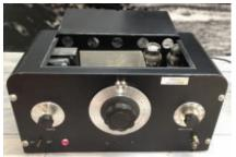
Fig. 2 Fully functional HP200A audio oscillator, the first product offered by HP.
