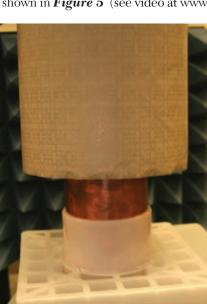
▲ Fig. 5 Placing the cloak over a metal cylinder (pipe) to be cloaked.
